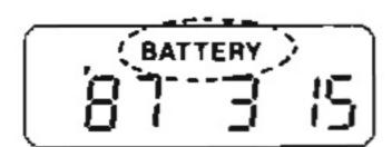
"Battery" appears to indicate that the battery should be replaced.
