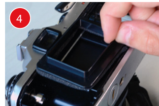
4 Centralize the gasket foam "C".
