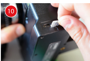
Insert the Micro SD card.
