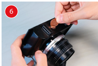
Screw the adapter with the help of a screwdriver or a coin.
