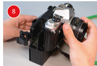
Slide the camera in the I'm Back 35 device and adjust the height of the focusing screen.
