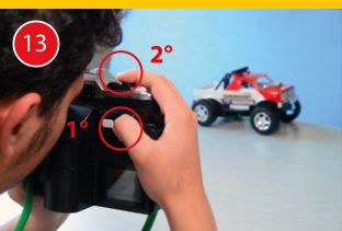
Click the "G" (OK) button first and then click the shutter button of the analog camera.
