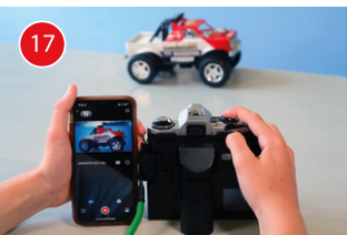
Open the I'm Back app and click "Connect Camera". This way you can view images directly to your smartphone.
