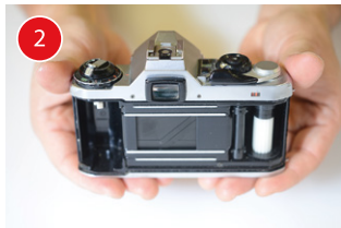
Remove the back cover.
