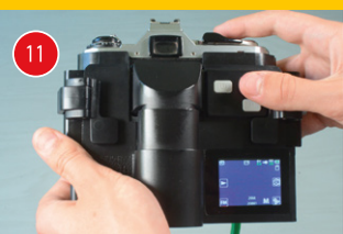
Turn on the I'm Back 35 by pressing the "F" button for 4 seconds. Format your SD card, clicking on the Tools icon and after "Format".
