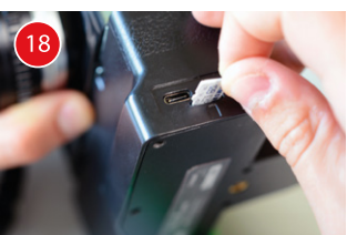
Remove the Micro SD to transfer the data to your computer, or connect the I'm Back 35 via the cable USB data.
