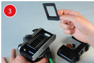
Carefully put the gasket foam "C" over the focal plane.
